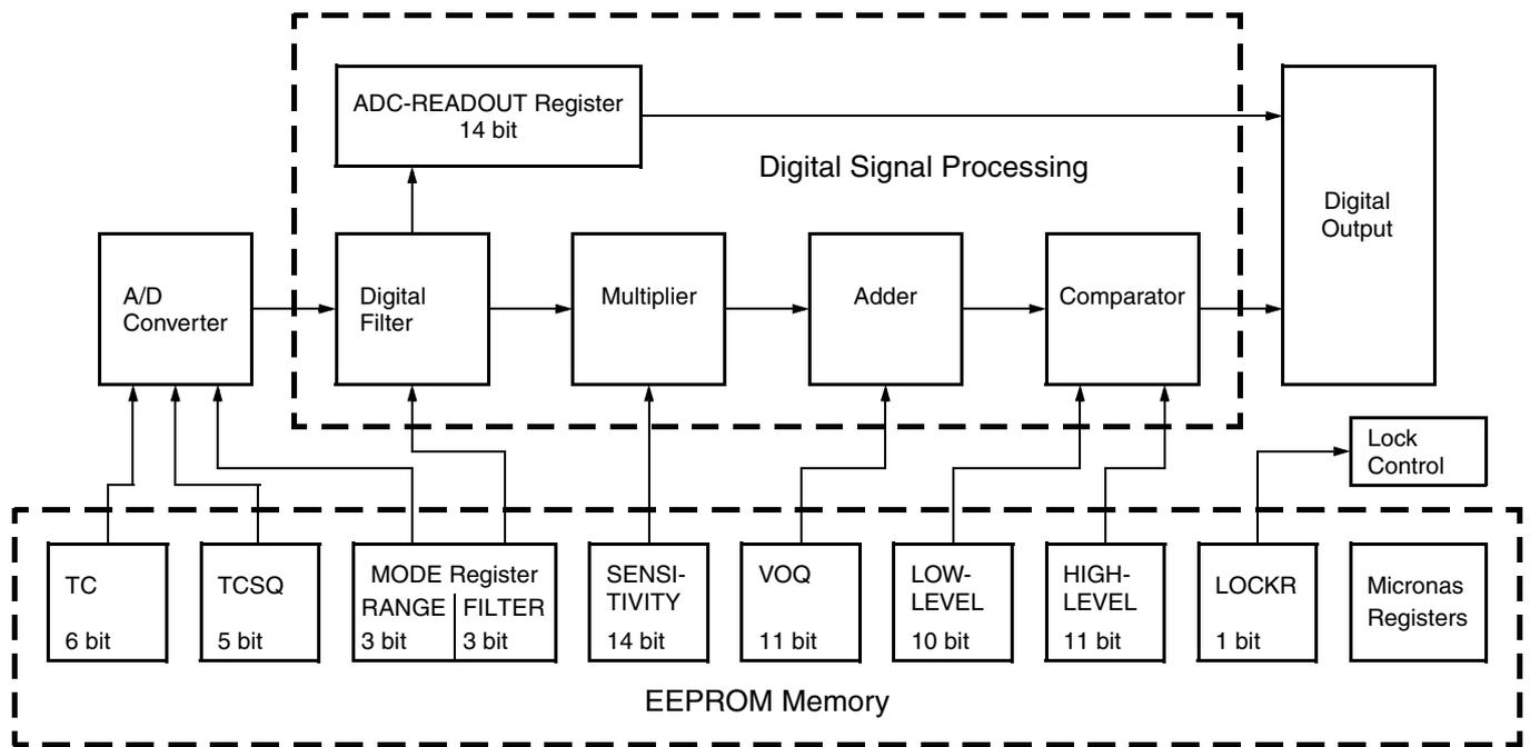
Fig. 2-3: Details of EEPROM and Digital Signal Processing
