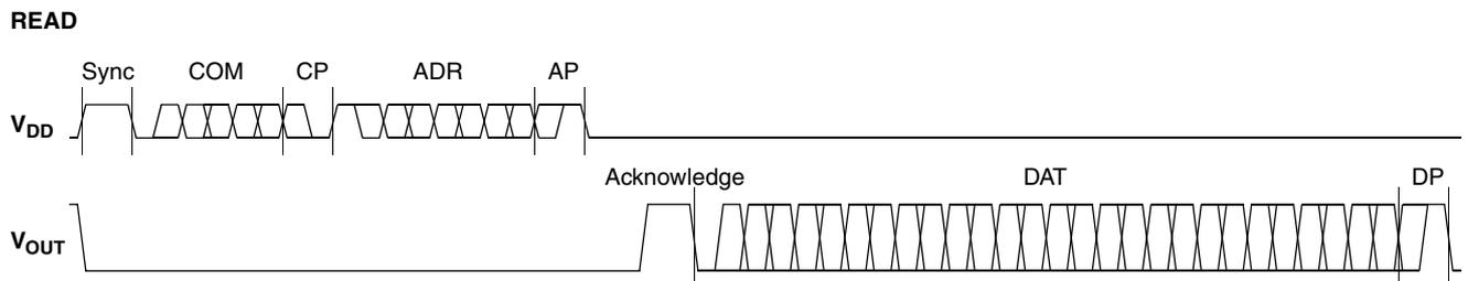
**Fig. 5-3:** Telegram for coding a Read command
