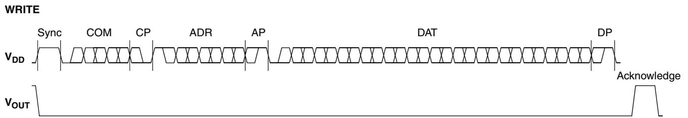
**Fig. 5-2:** Telegram for coding a Write command
