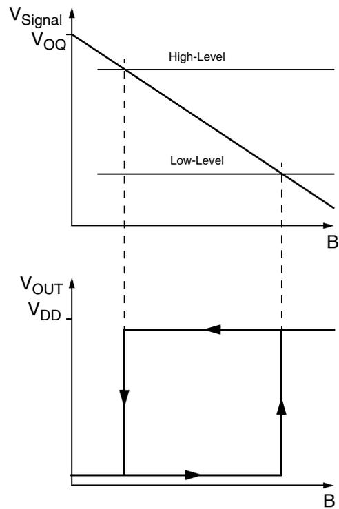
Fig. 2-6: HAL 1000 with unipolar inverted behavior
